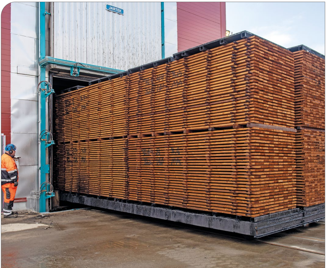
Figure 2. ThermoWood® being manufactured in process kiln.
