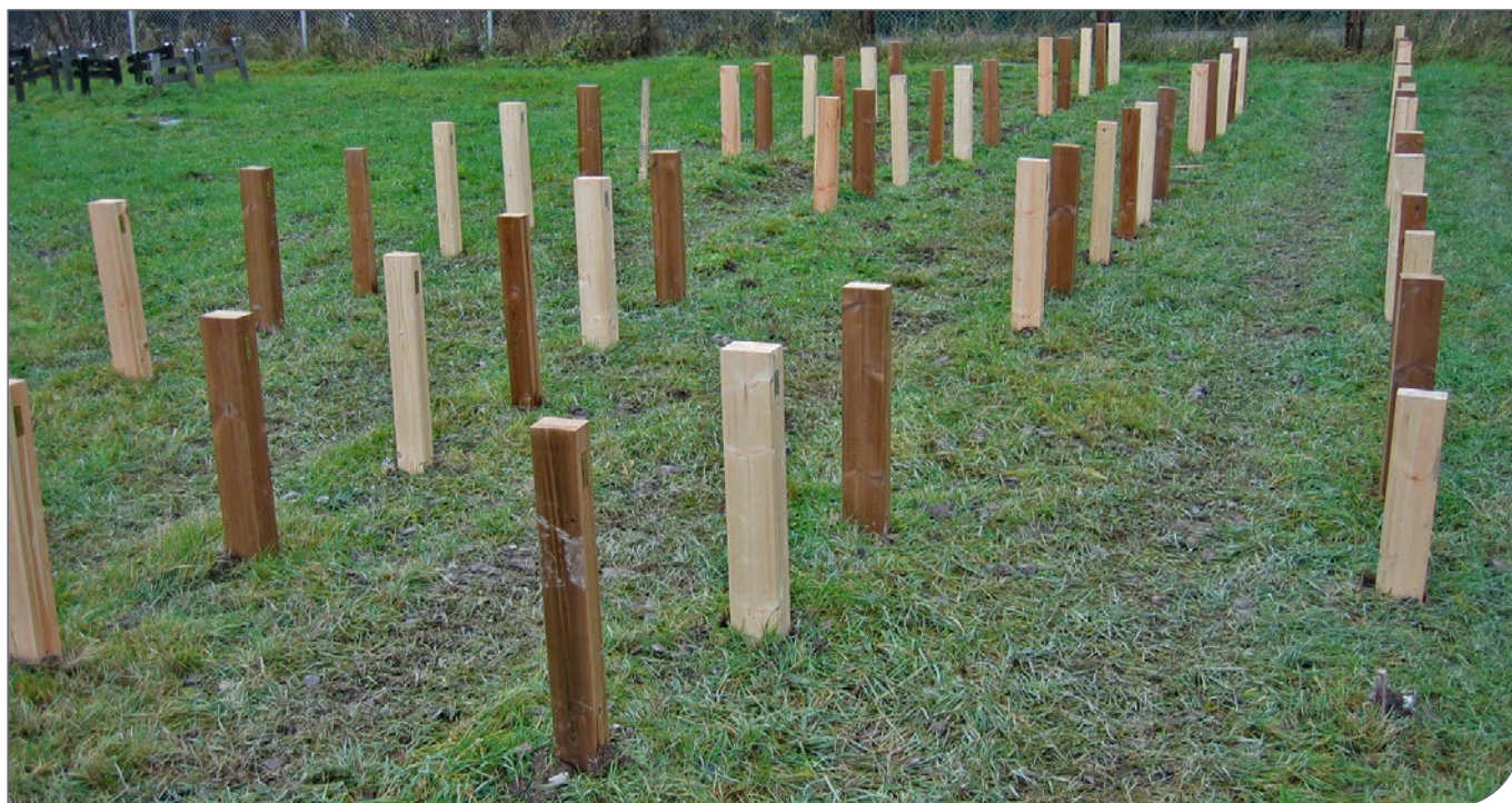
Figure 26. ThermoWood® field test in Espoo, Finland (VTT)
