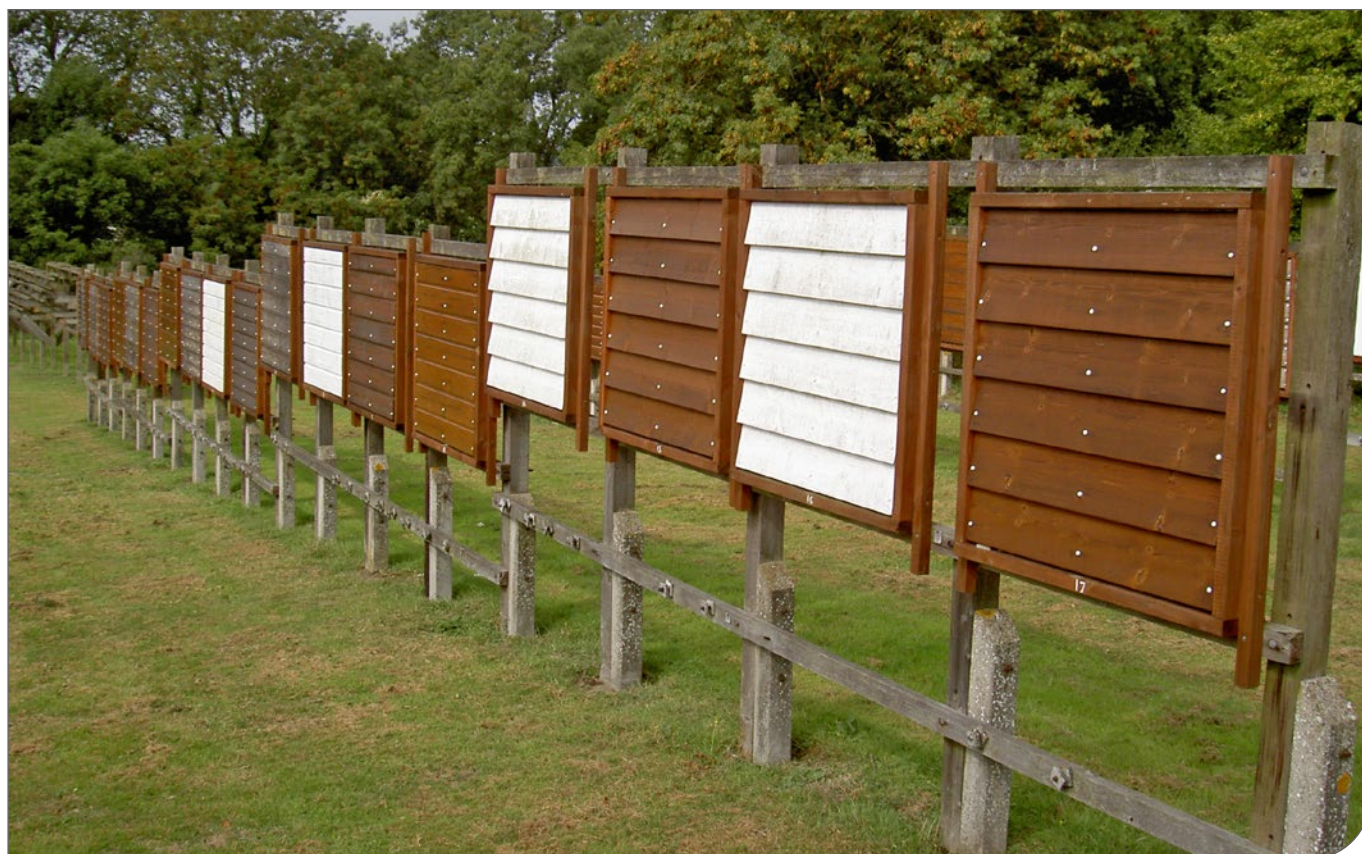
Figure 19. ThermoWood® field test in the UK (BRE).
